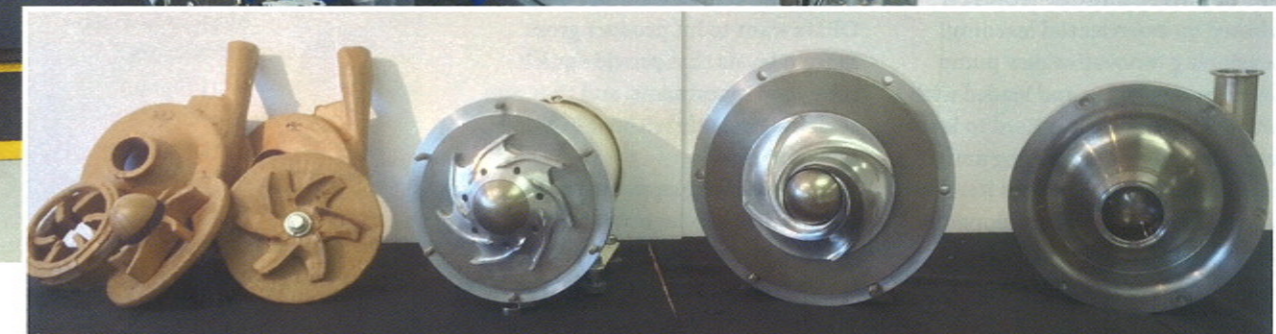
Image 3. Prototypes from four iterations involved in designing a sealless hygienic centrifugal pump. From left to right: cardboard and tape concept prototypes, aluminum concept prototype, aluminum functional prototype and stainless steel functional prototype
